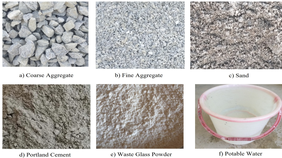
Figure 3. Materials for Concrete Mix Design
