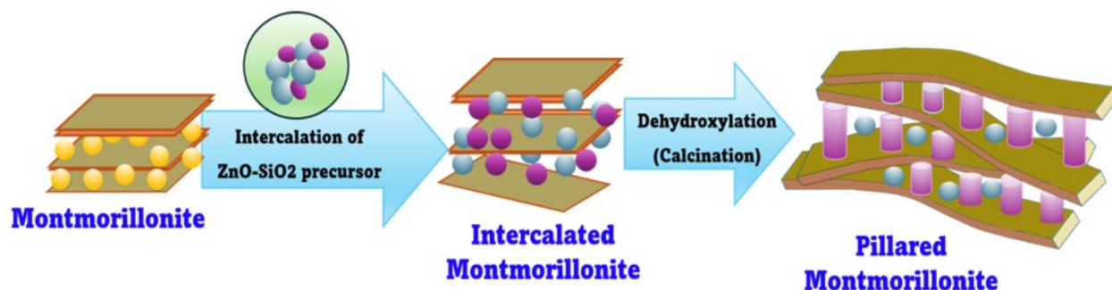
Figure 3. Schematic Representation of Pillarization and Formation of Uniform Interlayer's Distance
